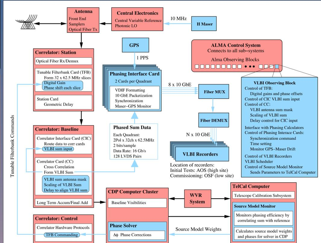
Fig. 4: The detailed design for the ALMA Beamformer. All blocks shown in orange are existing elements of the ALMA system, and blue blocks (and arrows) show elements of the Beamformer system.
