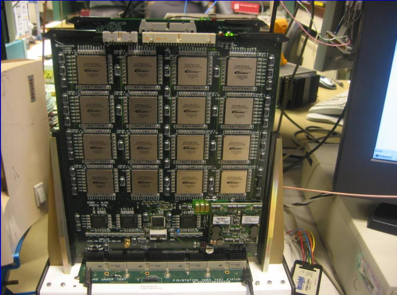
The TFB accepts a 2 GHz-wide digital signal and provides 32 independently tunable digital outputs, each filtered to a bandwidth of 62.5 MHz, which can be placed anywhere in the 2 GHz band. The outputs are sent for cross-correlation.
