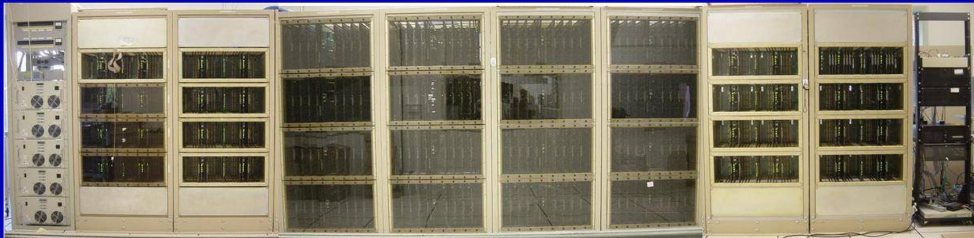
Complete correlator contains 2912 printed circuit boards and 5200 interface cables; there are more than 20 million solder joints.
